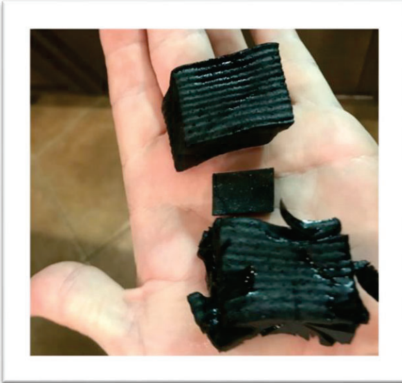
Figure 1- SwellFrac 400% Swell Out. All the samples shown were the same size
